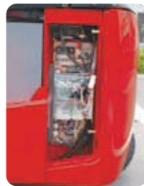
The controller is securely housed in the left side of the frame.
